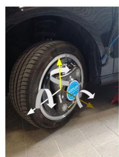
Wheel force reference sensor on the test vehicle
